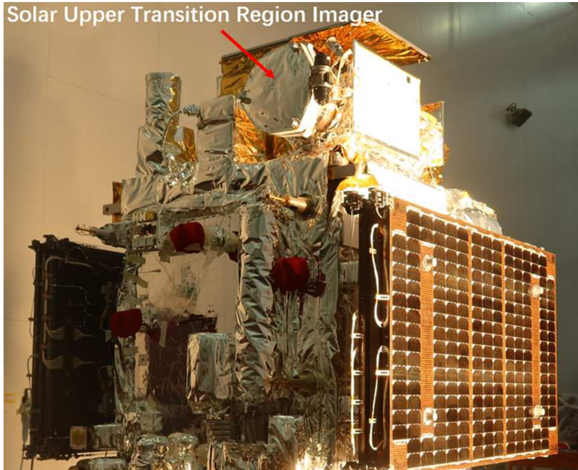
Fig. 6: SUTRI installed on the SATech-01 Satellite.
